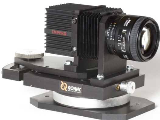
Camera on a mount for StereoPIV
